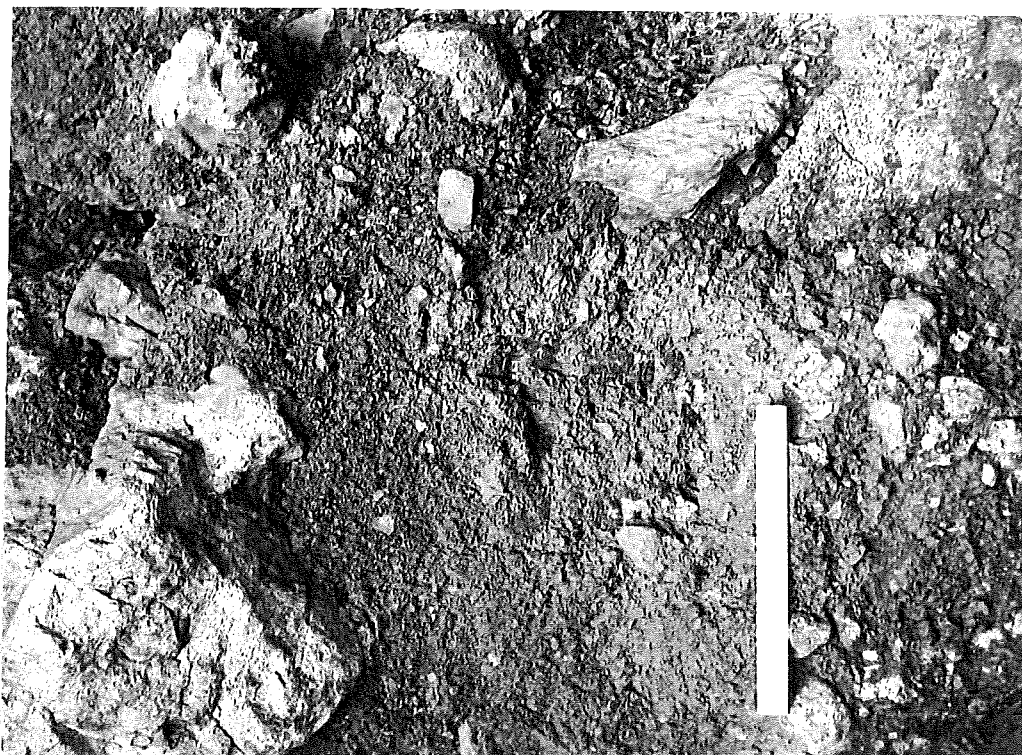
Plate IIa. Boulder colluvium at Mid-Levels, Hong Kong. A swirl structure related to material flow (screw) can be seen adjacent to the rule. Rule is 30.5 cm long.
